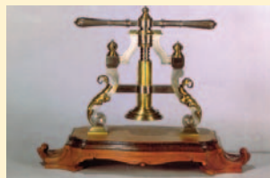
An instrument used to observe the porosity of materials, for instance iron and gold, which are the materials from which the sieves are made.
