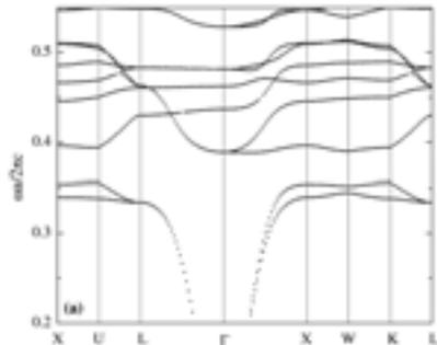
Calculated photonic band structures of a PC consisting of Te spheres in the fcc lattice with filling fraction 0.3. The extraordinary axis of Te spheres is oriented along [111]. A PBG between the second and third photonic bands can be seen with midgap ratio  $-\omega/\omega_c = 5.6\%$ , and a small PBG between the eighth and ninth photonic bands with  $-\omega/\omega_c = 0.84\%$ .
