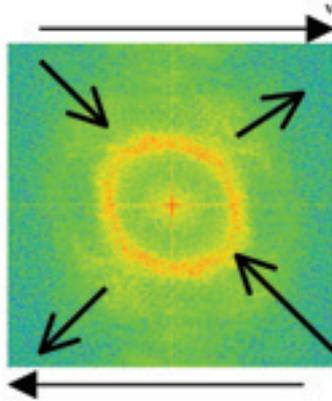
Schematic of the changes in the suspension microstructure as characterized by an FFT of an initially disordered suspension in the  $v-v$  plane at high  $Pe$  number. The arrows on the FFT indicate the compressional axis and the extensional axis of the flow field; the velocity vectors are drawn as well.
