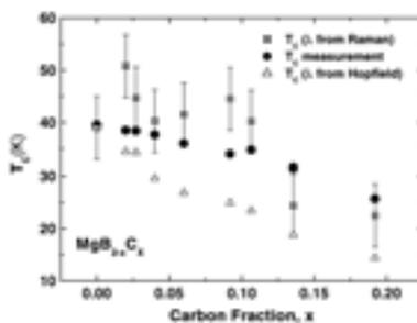
$T_C$  dependence on  $x$  in  $MgB_{2-x}C_x$ , calculated from the  $\lambda_{2g}$  variation obtained from Raman data, and from the Hopfield expression. The experimentally measured  $T_C$  is also shown for comparison.
