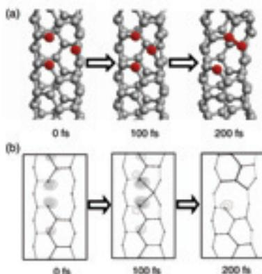
Self-healing process within a (3, 3) nanotube with a monatomic vacancy, induced by illumination. (a) Time evolution of the geometry. The three atoms adjacent to the vacancy and the new C–C bond, which forms  $\approx 200 \text{ fs}$  after the electronic excitation, are emphasized by colour and shading. (b) Time evolution of the partial charge density associated with the excited electron state. The lowest contour lines are common to the three panels.
