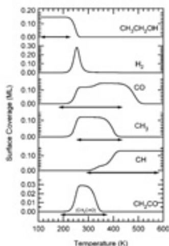
Surface concentration of the stable species during a simulated ethanol decomposition experiment on Pt(111), as a function of temperature, on the basis of the results obtained with the simple UBI-QEP model. Arrows indicate the temperature range in which the species are found to be stable on the basis of real time temperature-dependent XPS data
