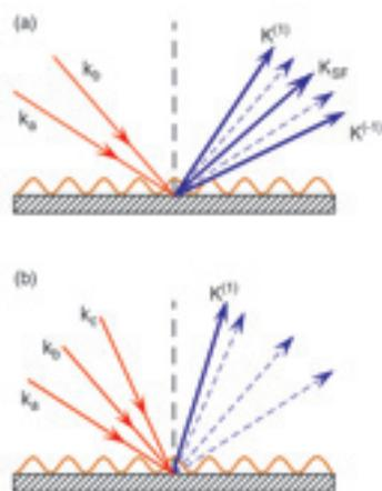
A schematic drawing of wave-mixing processes at surfaces in reflection geometry; (a) for two and (b) for three incident laser beams.
