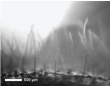
Optical micrograph of the hydrophobic polyether structure that was obtained by remoulding of the silicone elastomer, which was the direct mould of the lady's mantle leaf.
