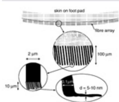
A schematic picture of the lizard adhesive system. The skin of the lizard is covered by a dense layer of thin fibres or hairs (setae; length:  $\approx 100 \mu\text{m}$  and thickness of fibre:  $\sim 4 \mu\text{m}$ ). Each of these fibres branches into about 1000 thinner fibres (length:  $\sim 10 \mu\text{m}$  and width:  $\sim 0.1 \mu\text{m}$ ). Each of the thin fibres ends with a thin (5–10 nm) leaf-like plate (spatula).
