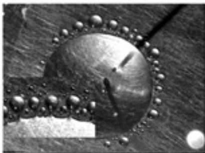
Contact line instability and emitted satellite droplets at high voltage. (Deionized water on silanized glass; droplet diameter:  $\approx 3$  mm.) Note the liquid necks between the satellites and the large droplet (inset).
