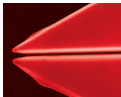
A nanofluidic emitter tip obtained by focused ion beam nanofabrication S Arscott and D Troadec 2005 Nanotechnology 16 2295–2302
